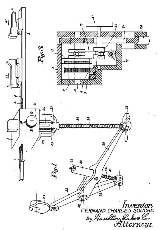
PUBLISHED JUNE 8, 1943. F. C. SOUCHE AUTOMATIC LINE CENTERING AND SHIFTING DEVICE FOR TYPE SETTING MACHINES Filed Oct. 15, 1942
