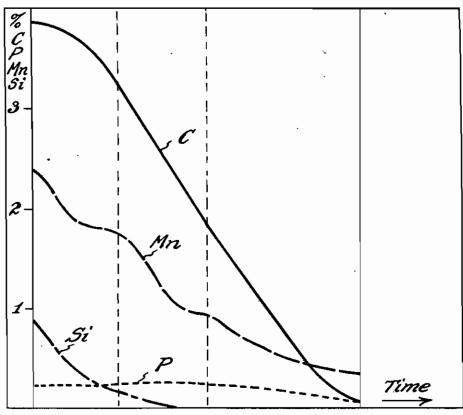
3.5% Scrap 2% Scrap 1.5% Scrap End of Charge 2.5% lime
